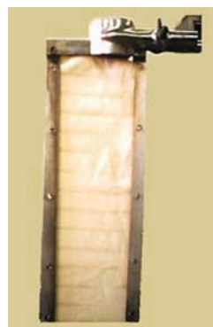
Fig. 1 Mostashari's flammability tester with an untreated cotton fabric before the accomplishment of the experiment
